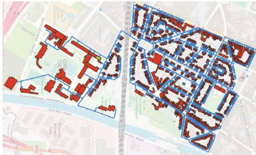
Figure 8: Full scenario (100% of the district is connected) simulated in nPro online tool
