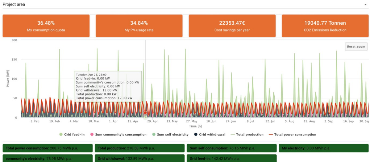
Figure 3: Building power calculations of Kahlenbergdorf DH
